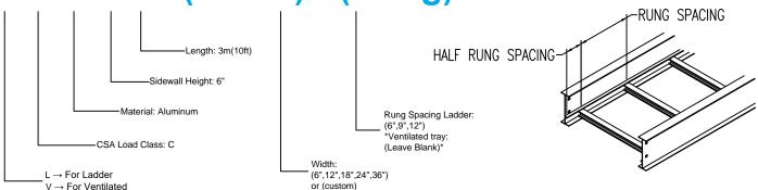
\* CSA Ventilated tray has a rung spacing of 4" between rungs.
