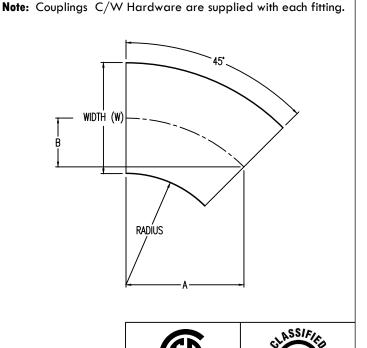
STEEL LADDER/VENTILATED TRAY HORIZONTAL 45° ELBOW ORDERING DATA EXAMPLE
